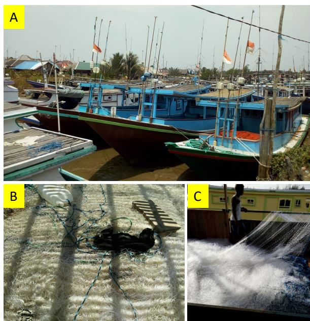
Fig. 2. Characteristics of (A) the fishing fleets of 18–21 GT, (B–C) the gillnets for Scomberomorus commerson and S. guttatus made of PA monofilament with 4 and 2¼ inches stretched mesh sizes, respectively used in Tanah Laut District, South Kalimantan, Indonesia.
